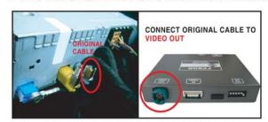
1) CONNECT ORIGINAL CABLE TO AUDI INTERFACE BODY [ VIDEO OUT ] SOCKET.
