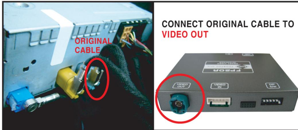
1) CONNECT ORIGINAL CABLE TO AUDI INTERFACE BODY [ VIDEO OUT ] SOCKET.
