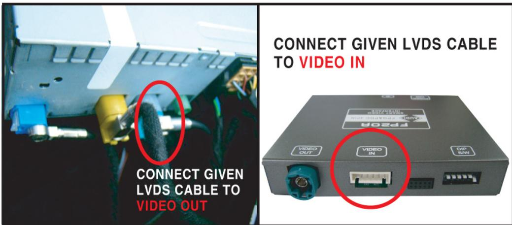
2) CONNECT GIVEN LVDS CABLE TO BOTH AUDI ORIGINAL SOCKET AND AUDI INTERFACE BODY [ VIDEO IN ] SOCKET.
