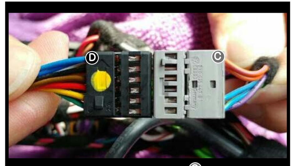
4. PLEASE USE REMOVED OEM CONNECTOR **(C)** CONNECT WITH **(D)** AS PICTURE SHOWN.
