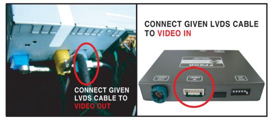
2) CONNECT GIVEN LVDS CABLE TO BOTH AUDI ORIGINAL SOCKET AND AUDI INTERFACE BODY [ VIDEO IN ]SOCKET.
