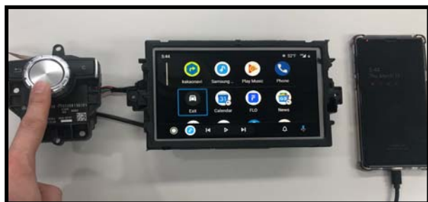
SELECT "EXIT" OF ANDROID AUTO AND PRESS ENTER" TO MAIN MENU OF NETPLAY
